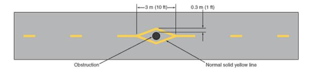
Markings as shown above should also be used at the location of obstructions in the center of the path, including vertical elements such as bollards, intended to physically prevent unauthorized motor vehicles from entering the path.
