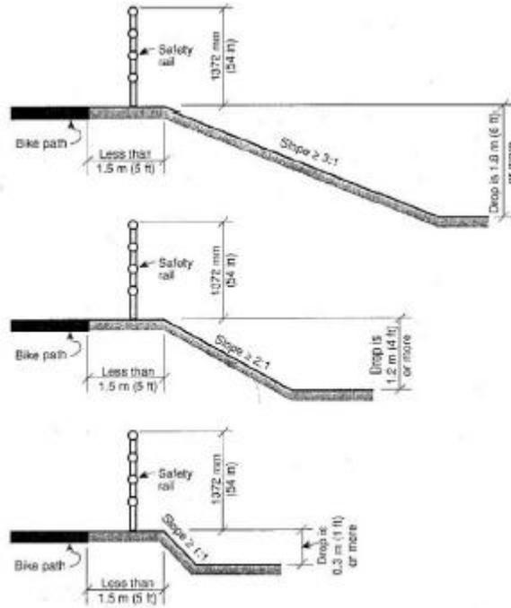
**Figure 10: Connecticut Identification of Drop-Off Hazards (5)**
